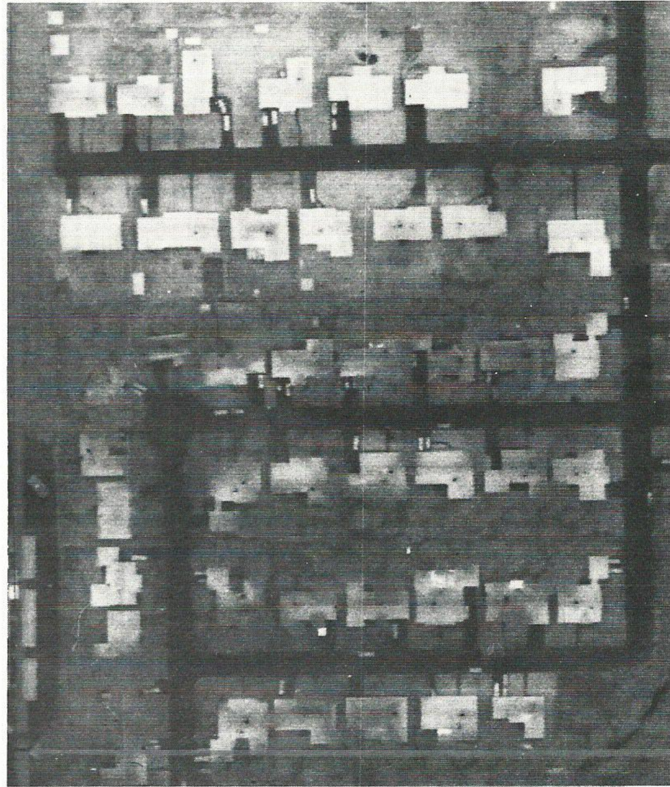
Infrared photography used to detect heat loss
