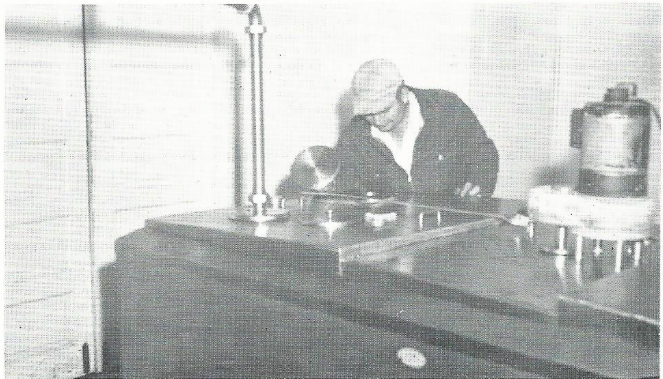
MILK STORAGE. Herd Manager Sam Morris checks the bulk milk cooler. Later, milk will be pumped electrically into tank truck to be hauled to the Kleinpeter Farms Dairy for processing.
