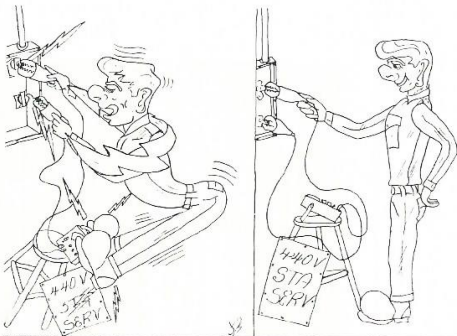
Never Use Both Hands to Hold Test Clips While Testing Voltage, Etc.
