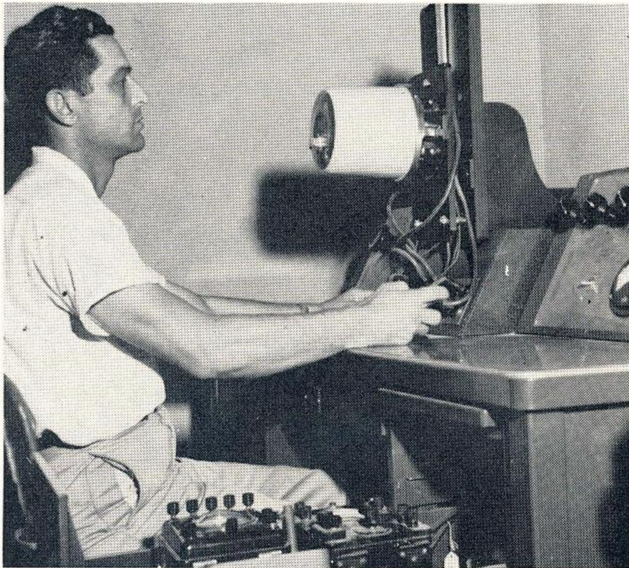
Load meters are also tested on this testing board. Here, Lee Broussard tests a meter on full load and light load. The primary standard at his right leg indicates the accuracy of the meter being tested. Life of a meter is usually 30 years, although most will last even longer.
