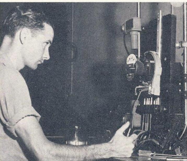
After being cleaned and having jewels replaced, meters are ready for testing and are placed on the test board at left. Here, Victor Netteville, shop and field tester, tests a residential meter on full load—equivalent to all appliances in a home going at once—then on light load. Accuracy of Gulf States’ meters varies only one-half of one per cent before they are installed.
