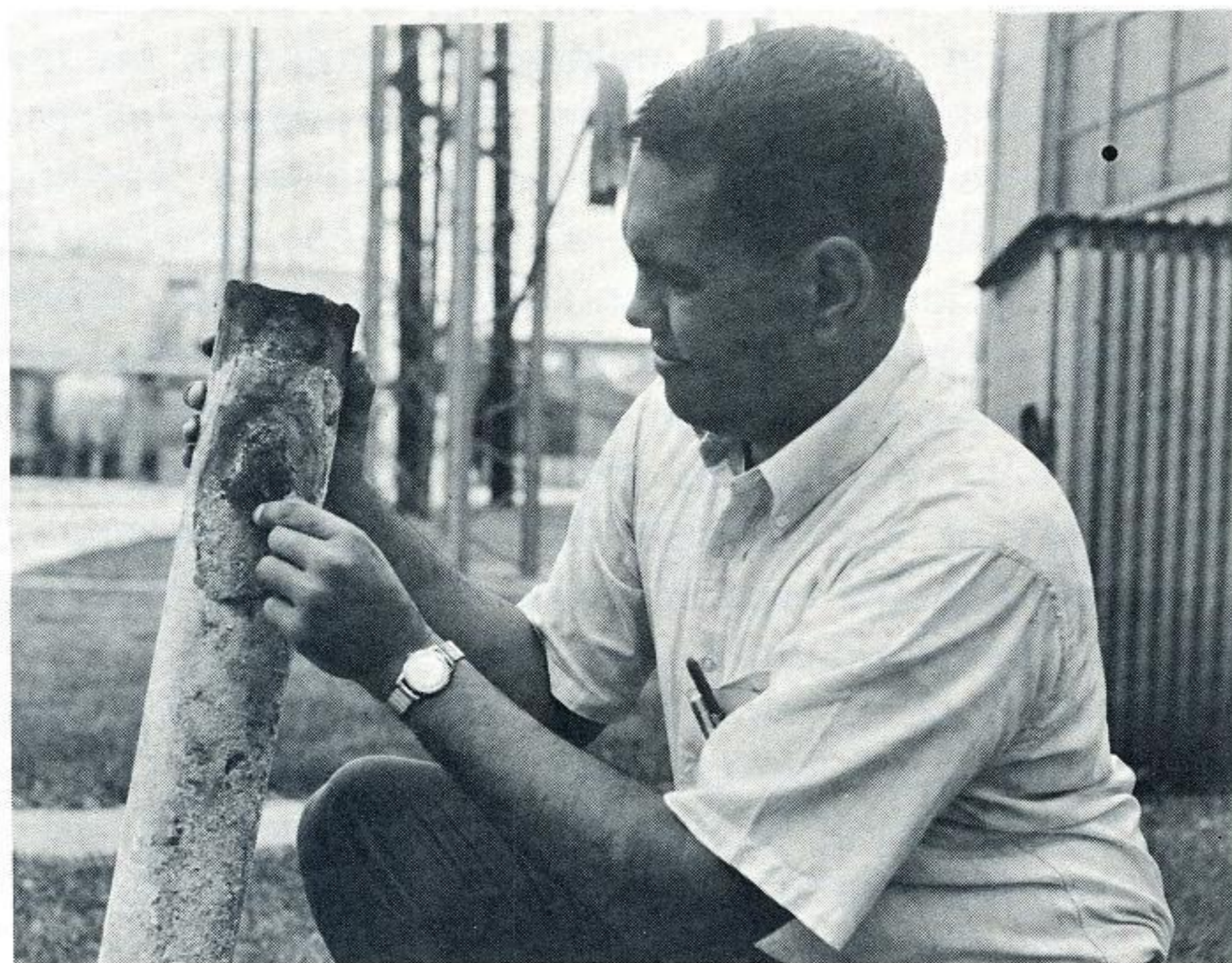
Weldon Smith , chemist at Louisiana Station, points to rupture in boiler tube caused by calcium carbonate buildup. Hole allows water to escape and eventually starves a tube.
