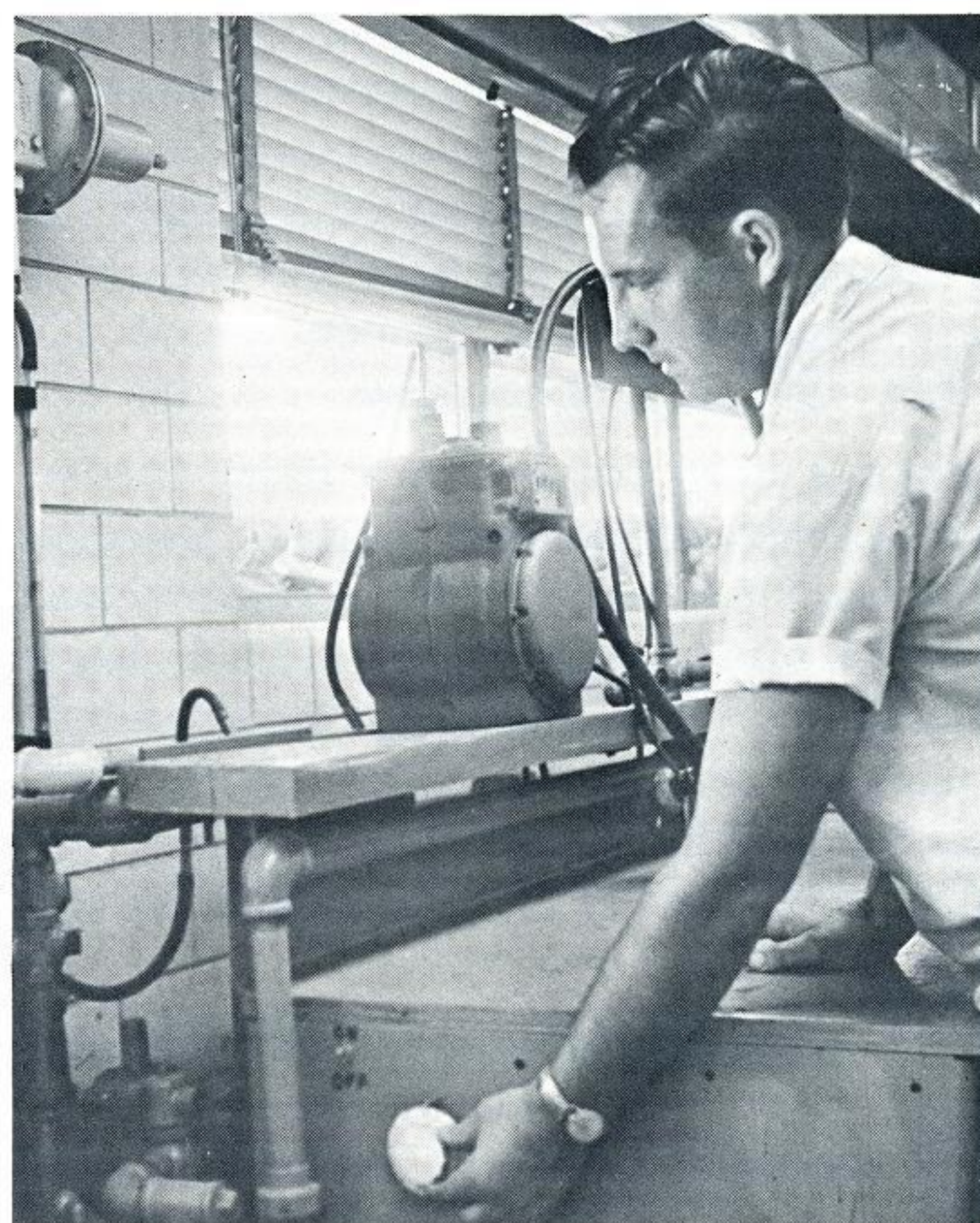
Aubrey Lee , meterman, sets homemade timer which tests meters for very small leaks. The timer control is off of a washing machine; the manifold was also built in the Meter Department.
