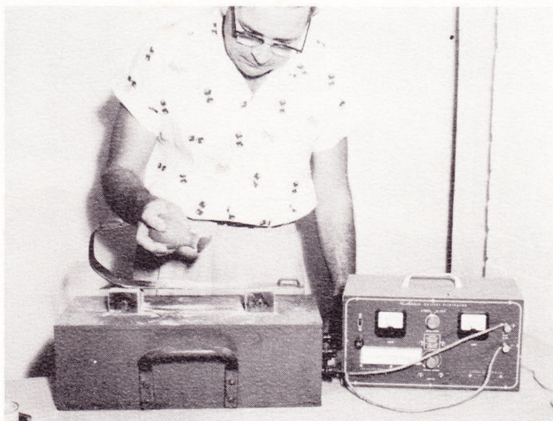
W. L. Parker is shown using the climbing tool tester which was developed by Louisiana Station employees.
