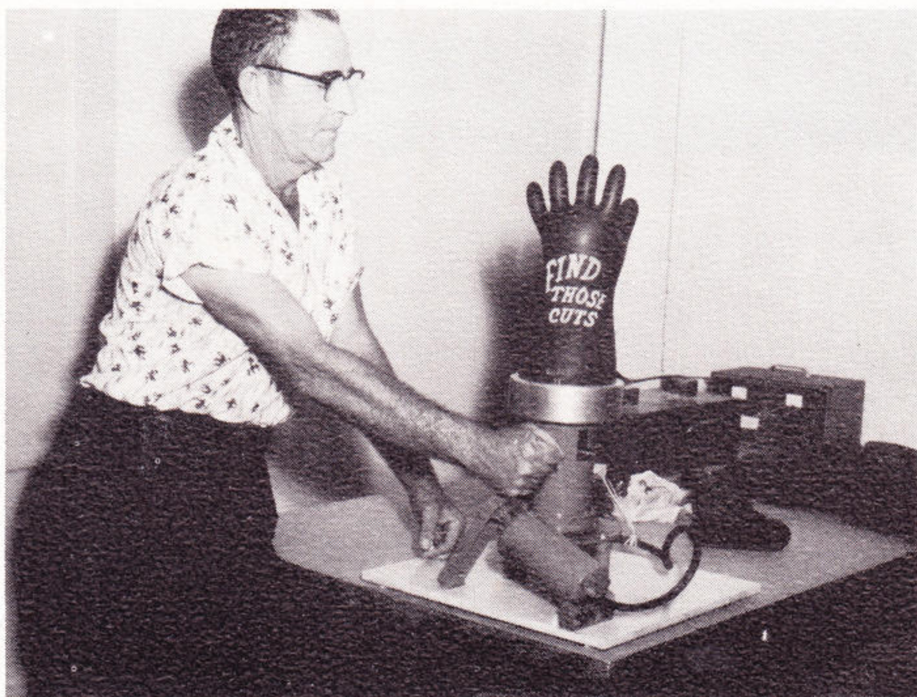
M. C. Akins demonstrates the tester for linemen's rubber gloves which was designed by Company employees.
